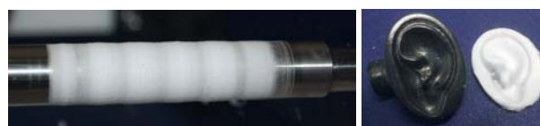
Fig. 1: Left: Electrospun trachea-like construct by using a user-defined speed profile of the mandrel. Right: Electrospun ear-shape and its mould after de-moulding
