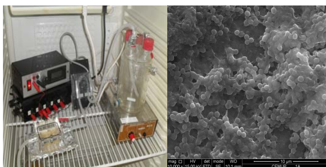
Fig. 1: Photograph of the experimental system used to perform biofilm formation on the reactor. And SEM micrographics of biofilms grown on nanoHA disks collected at 30000 magnifications, with a working distance of 10 mm and an x-ray energy of 15 kV. Where a mature biofilm embedded in an extracellular matrix was observed.
